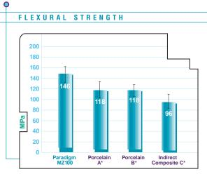
The 3M<sup>™</sup> Paradigm<sup>™</sup> MZ100 Block for CEREC<sup>®</sup> offers higher flexural strength than that of porcelain blocks available today (A & B) or indirect composite (C).
