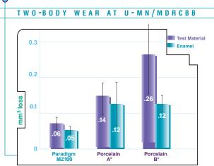
The 3M<sup>™</sup> Paradigm<sup>™</sup> MZ100 Block for CEREC<sup>®</sup> exhibited less wear than porcelain blocks (A & B) in a two-body wear study.
