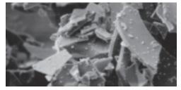
Large cleaning particles within the paste (magnified 3000x) break into fine polishing particles in a matter of seconds.
