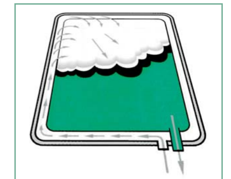
Schematic of forced air removal design with combined purging
