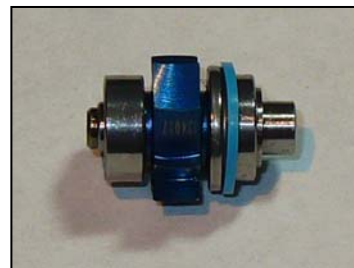
2 Place blue o-ring on front bearing of turbine assembly
