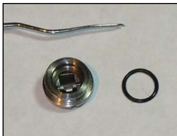
1 Place black o-ring into back cap
