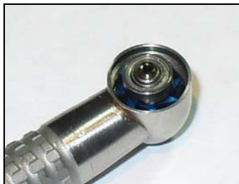
3 Insert turbine assembly into head housing
