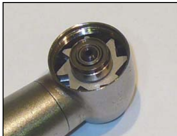
3 Insert turbine assembly into head housing
