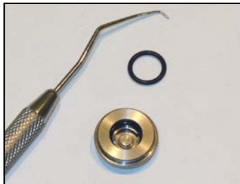
1 Place o-ring into back cap
