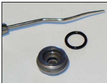
1 Place o-ring into back cap
