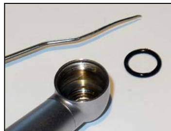
2 Place o-ring into head housing
