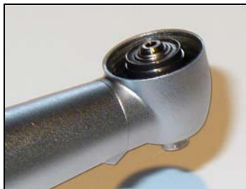
3 Insert turbine assembly into head housing
