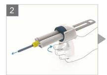
Pull the trigger until the material is coming out.
