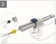
Remove cap and attach mixing tip. Note the corresponding notches.
