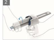
Lock the cartridge by turning it by 90° counter-clockwise.
