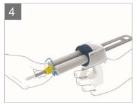
Turn the mixing tip by 90° clockwise to lock it.
