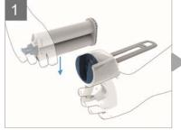
Insert the cartridge into the rotation ring – slim side downward (not relevant for 1:1 cartridges).
