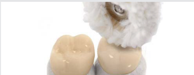
150: High gloss polishing of the crown with a cotton buff, Recommended rotary speed: 7.000 - 12.000 rpm
