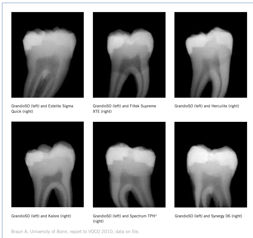
X-rays of GrandioSO and other composites. Showing differences in radiopacity.
