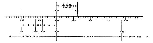
Visible-light-cured dental restorative resins are hardened only by light at the blue end of the visible spectrum. The wavelength range for activation is 400 nm to 520 nm, which includes the blue spectrum. The design of the DIGITAL LIGHT METER – 200 is versatile and can be used for various requirements.
