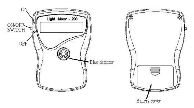
Tune power on. Then you can measure the light intensity of blue light used for curing. Align the tip of the light guide to the aperture window. Position your curing light guide so that the light is perpendicular the window. Read the output directly on the meter.
