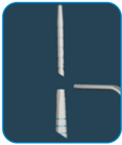
Remove the set, wipe them separately with alcohol and air jets
