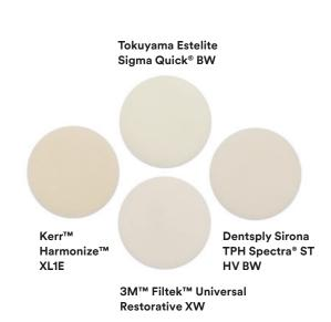
In the graph to the left, we measured W\* values, which are the values of whiteness of a material. As a material becomes "whiter," its W\* value approaches zero. Pure white (W\* = 0) is used as a reference for the test data. 3M<sup>™</sup> Filtek<sup>™</sup> Universal is significantly whiter in color than Tokuyama Estelite Sigma Quick<sup>®</sup> BW, Kerr<sup>™</sup> Harmonize<sup>™</sup> XL1E and Dentsply Sirona TPH Spectra<sup>®</sup> ST HV BW.
