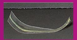
A traditional monomer containing composites cured in a thin film. The resulting shrinkage curls the thin film.
