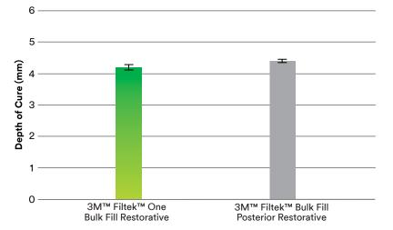
Figure 8: ISO 4049 Depth of Cure – 3M<sup>™</sup> Filtek<sup>™</sup> One Bulk Fill Restorative and 3M<sup>™</sup> Filtek<sup>™</sup> Bulk Fill Posterior Restorative. 20-second exposure, 3M<sup>™</sup> Elipar<sup>™</sup> DeepCure-S LED Curing Light. *Source: 3M internal data*
