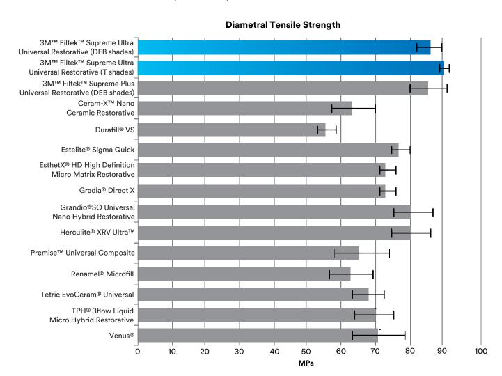
Diametral tensile strength. Source: 3M internal data
