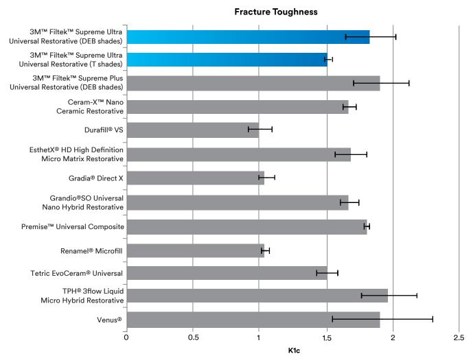
Fracture toughness. Source: 3M internal data
