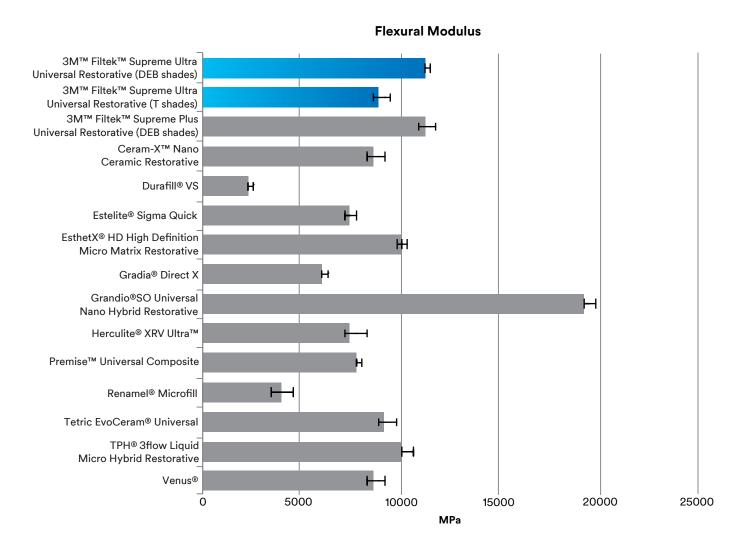
Flexural modulus. Source: 3M internal data
