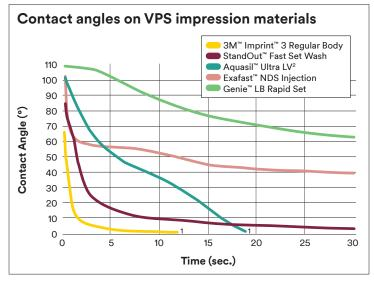
Fig. 1: More hydrophilic: 3M<sup>™</sup> Imprint<sup>™</sup> 3 Regular Body VPS Impression Material has one of the lowest contact angles tested on set VPS impression materials. Source: 3M internal data.
