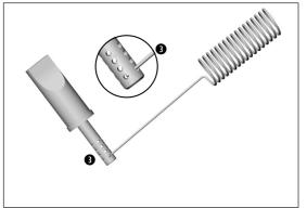
3 Clean outlets carefully with the cleaning wire to remove dirt and deposits.
