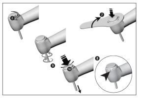
Screw the push-button onto the turbine head.
