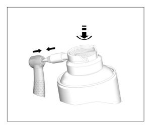
Lubrication of the chucking system
