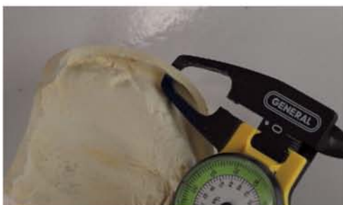
Fig. N The width of the land area should be 3-4 mm.
