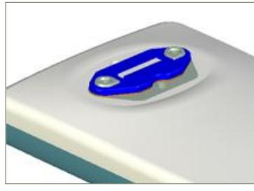
Using tweezers, remove the small elastomer strip from the Sensor. **Do not remove frame**. Dispose of this strip, as it will be replaced.
