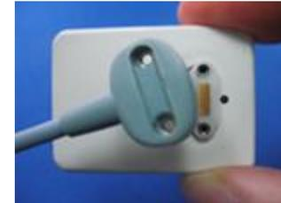
Remove cable from kit. Align the cable to the Sensor (sample shown) so the Sensor keying feature connects to the corresponding key in the cable. When properly aligned, the cable fits the back of the Sensor evenly and the metal area is completely covered.
