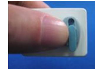
Remove cable from kit. Align the cable to the Sensor (sample shown) so the Sensor keying feature connects to the corresponding key in the cable. When properly aligned, the cable fits the back of the Sensor evenly and the metal area is completely covered.
