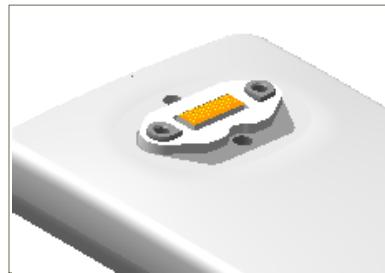
Using fingers, remove the small frame with elastomer strip from the Sensor. Dispose of this part, as it will be replaced.
