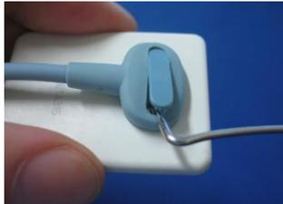
Using a dental instrument, carefully lift and remove the tab cover from the back of the Sensor cable. Dispose of the tab cover as a new one will be used when the new cable is attached.
