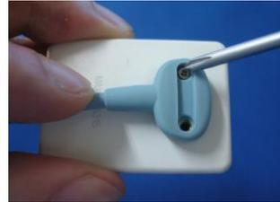
Using the screwdriver provided, loosen and remove the 2 screws that secure the cable to the Sensor. *If silicone gel is present, remove this material and discard it.* Dispose of the screws as new ones are supplied. Remove the cable from the Sensor.
